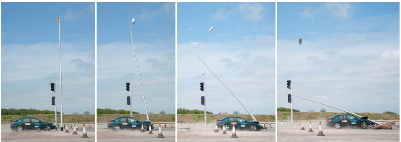
Crash test (demonstration) HE-C pole
