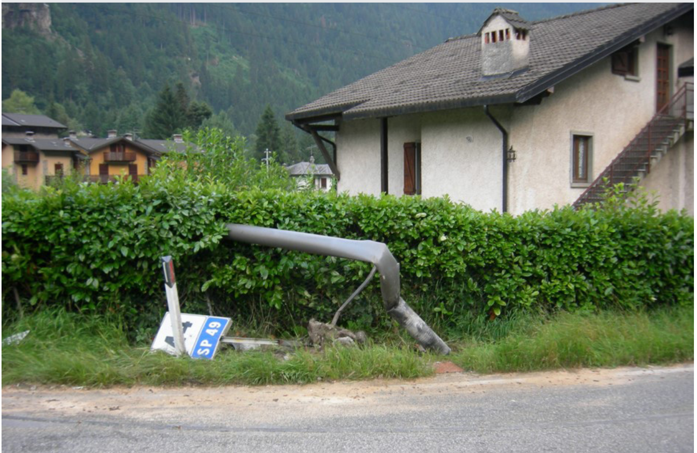
LE-C aluminium light pole crashed in the province of Bergamo, Italy
