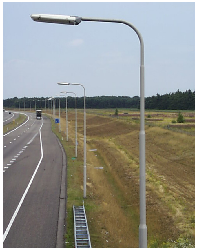
There is less danger behind the pole. A crash barrier is not necessary if the pole is passive safe.
