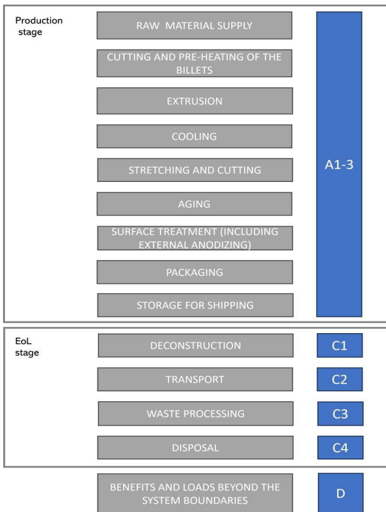
Figure 1. Scheme of the profiles manufacturing process occurring at Mississauga
